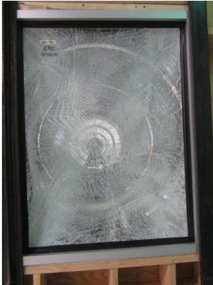
Photo No. 12 Post-test Specimen #4, Interior
