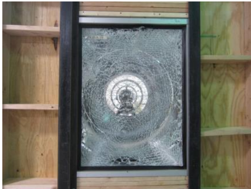
Photo No. 14 Post-test Specimen #5, Interior
